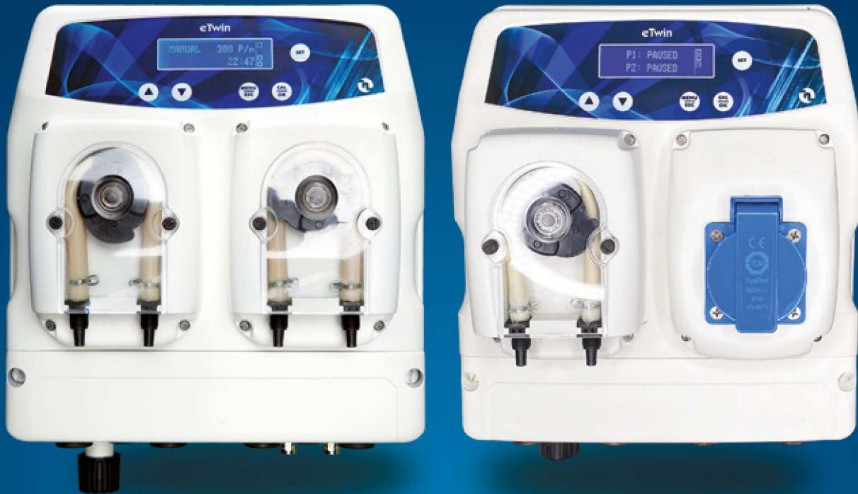
The eTwin is a compact, easy-to-use equipment consisting of two dosing pumps and two parameters controllers designed to measure pH, Redox and Chlorine plus the temperature. Mainly conceived for pool's industry, the dosing pumps are available either in peristaltic and solenoid versions.
